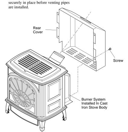
Figure 17 - Installing Rear Cover
